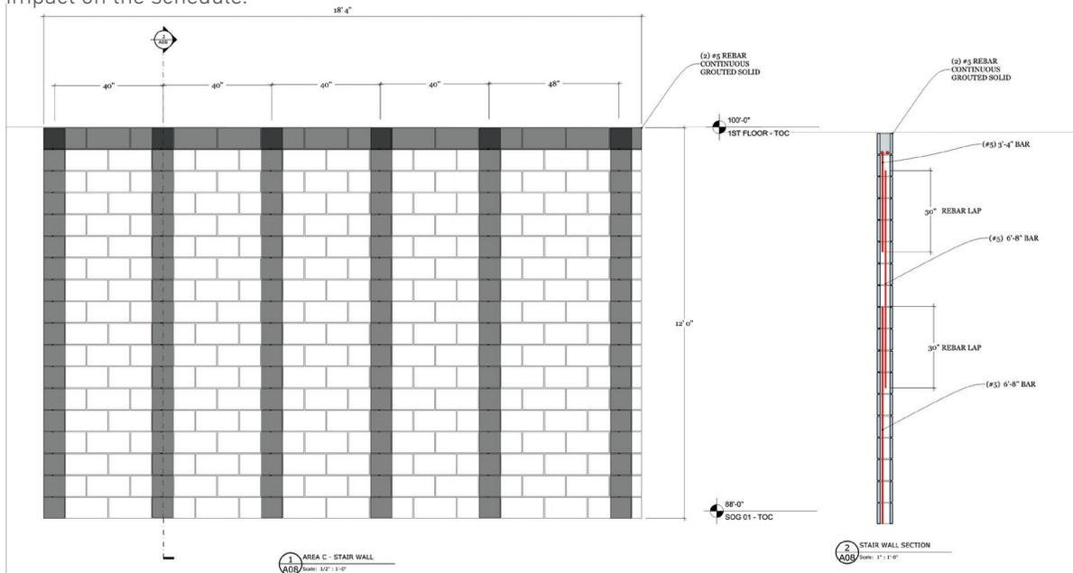
**Figure 9: St. Augustine 2D lift drawing showing grout, rebar and bond beam locations generated from 3D SketchUp model**
