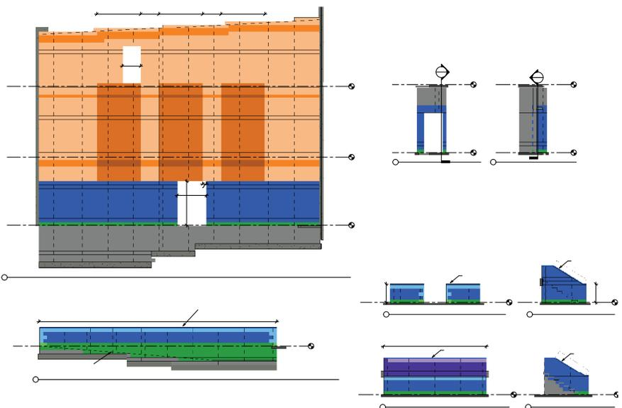
Figure 5: Washington High School 2D lift drawing showing CMU types and layout generated from Revit model
