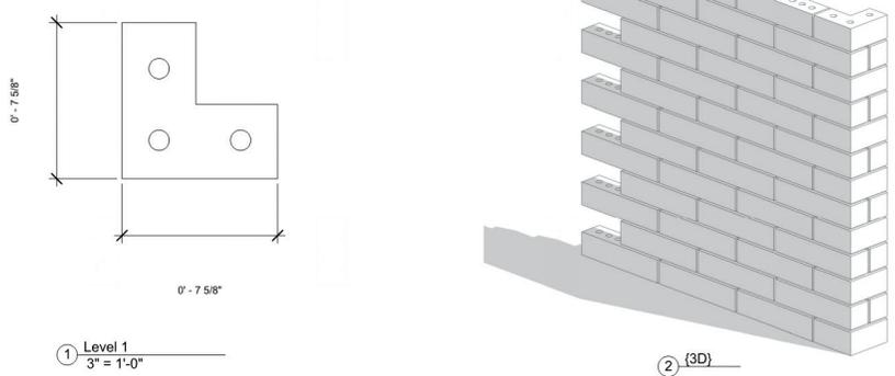
Figure 3: Occhiato University Center shop drawing of special shape return brick generated by Revit model
