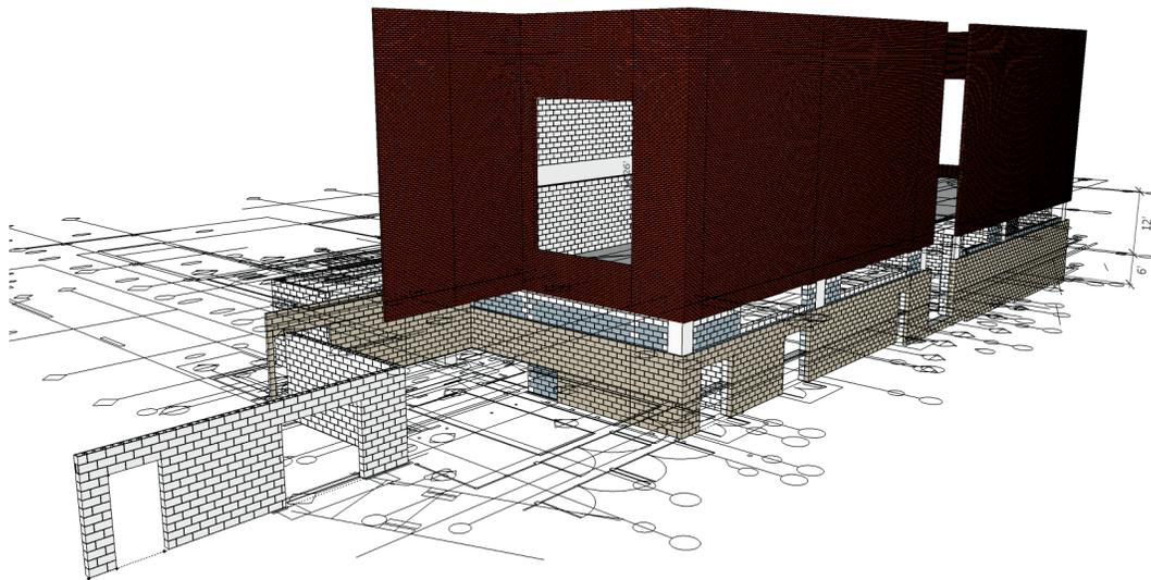
**Figure 7:** WMH 3D SketchUp model showing Burnished CMU, Brick and CMU back up shows layout and bond
